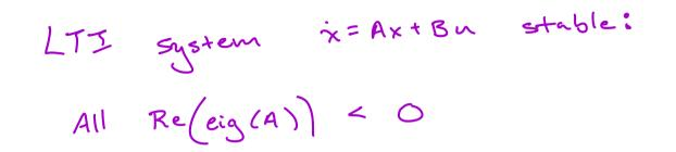
Stabilizable if H is controllable in the direction of the eigenvectors w/ nonnegative eigenvalues
