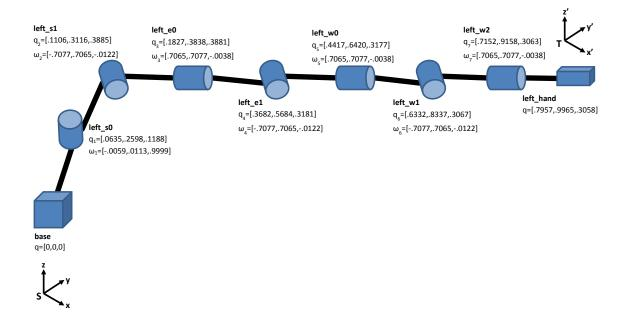
Figure 1: Example robot arm parameters (Baxter).
