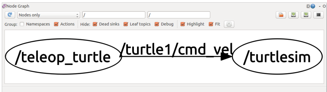
Figure 3: Output of rqt_graph when running turtlesim .
