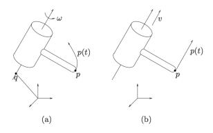
Figure 3: a) A revolute joint and b) a prismatic joint.
