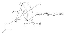
Figure 4: Generalized screw motion.
