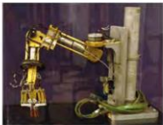
Figure 1.50: Stanford University(1963): Rancho Arm, the first artificial robotic arm to be controlled by a computer.
