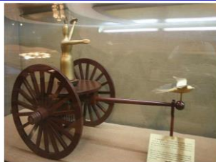
Figure 1.6: Zhang Heng (100 A.D.): South-pointing Chariot (non-magnetic differential mechanism)
