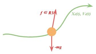
Above: By treating the quadrotor as a single point mass, we can easily develop a position controller.
