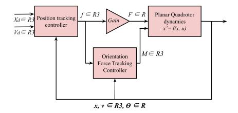
Notice the "cascaded" structure of the two feedback controllers, where the output of one controller is passed into the next. The control inputs to this system are a total thrust force  $F \in \mathbb{R}$  and moment  $M \in \mathbb{R}$  produced by the propellers.
