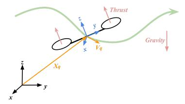
Imagine that we want to design a feedback controller for a simple *planar* quadrotor, which is constrained to travel and rotate in the XY plane. Our controller should track a trajectory  $x_d \in \mathbb{R}^3$  and provide stable flight. To accomplish these objectives simultaneously, we split our controller into stages.
