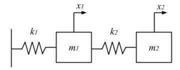
The springs have constants  $k_1$  and  $k_2$  and the masses have positions  $x_1$  and  $x_2$ . Assuming  $x_1$  and  $x_2$  are zero when the springs are unstretched, find the set of second order differential equations describing the motion of the masses. You may use either a Newtonian or Lagrangian approach. Assume that there are no frictional or gravitational forces.
