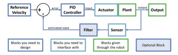
Figure 1: Block diagram of control scheme to be implemented.
