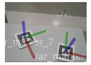
Figure 5: Tracking AR Tags with webcam
