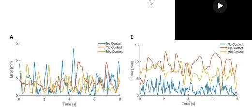
Fig. 4. Error plots for tracking. (A) With the soft cPDMS sensor. (B) With the commercial flex sensor.
