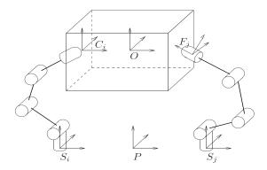
A multi-fingered robot hand has k fingers with joint angles  $\theta_{f_1}, \ldots \theta_{f_k} \in \Re^n$  Each of the fingers is a robot in its own right so the composite dynamics are
