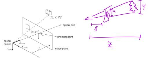
**Problem 5:** Using the image above, find the relationship between the 3D point  $(X, Y, Z)^T$  to its corresponding 2D projection (u, v) onto the imaging plane (assume the focal length is 1).
